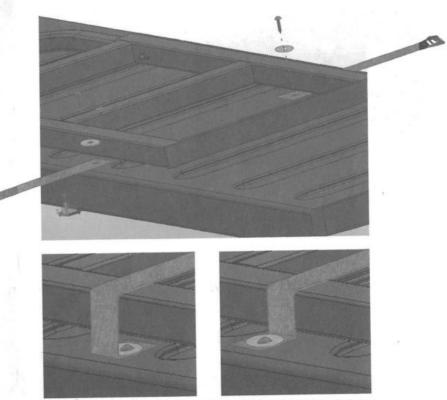
Secure straps in either direction as needed with your specific tailgate.
