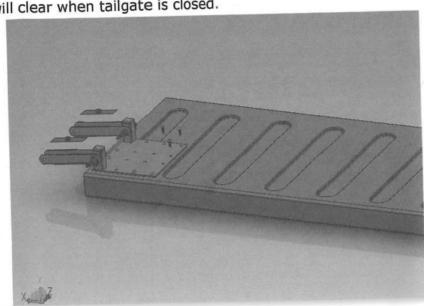
NOTE: Only half of the holes in the mounting plate will be used. Based on model of truck/tailgate the screw hole locations will vary. Optimum screw locations are the front and back sides of mounting plate - instead of the interior holes.
