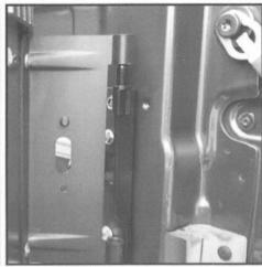
a.Clasp the storage tool box onto the two Hinge Pins of Bracket-2; b.Push the storage tool box to the stowed position.
