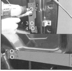
a. Fasten 1 Torx Bolt to the first screw on Bracket-2 first; b.Tighten the brackets with 5 Torx Bolts from 2 to 6.
